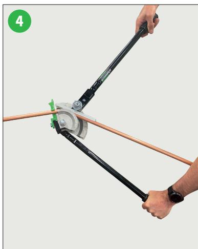
4 Holding one arm in each hand, bend the pipe (4, 5, 6, 7 and 8)
