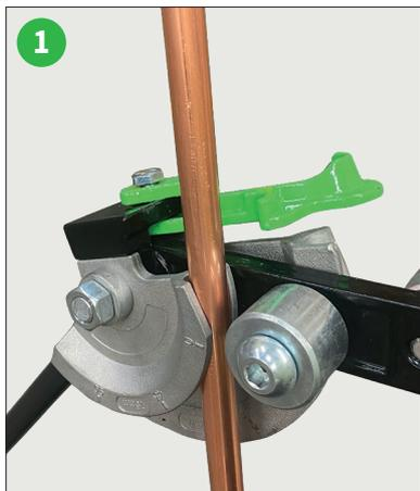
1 Place pipe between roller and former disc
