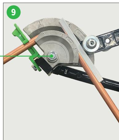
9 Use the 45° and 90° markers on the former disc as a guide when bending
